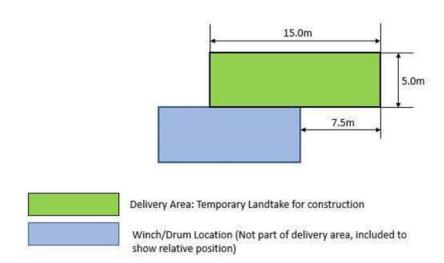
Example of single JB area during construction including laydown area on the side of the road
